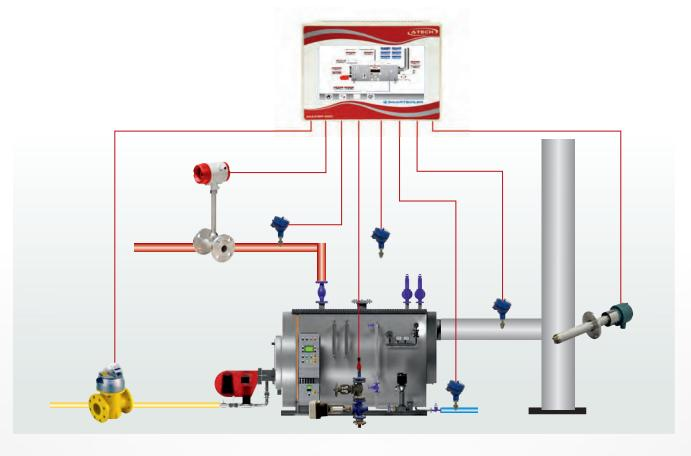
SmartEff 2000 Efficiency Monitoring System for steam boiler is a complete efficiency monitoring and analysis system for boilers. Continuous monitoring of performance parameters for prompt actions to improve boiler efficiency with direct or indirect method.
