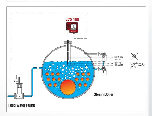
Two equipments are together in one compact system. Thus, no external control device is required.
